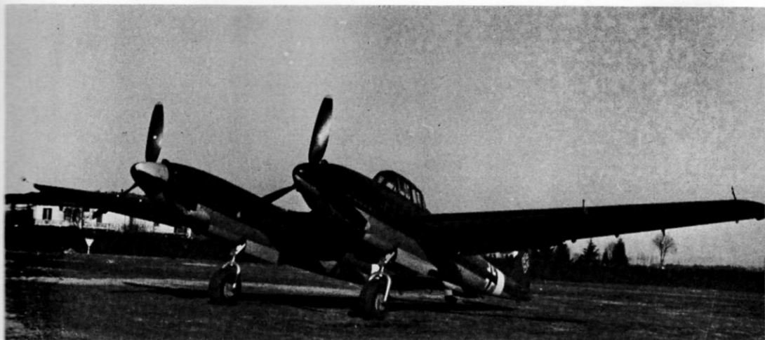
Savoia-Marchetti SM.92 heavy fighter prototype in Luftwaffe markings. This twin-boom design had a cockpit on the port fuselage only SIAI-Marchetti archives
