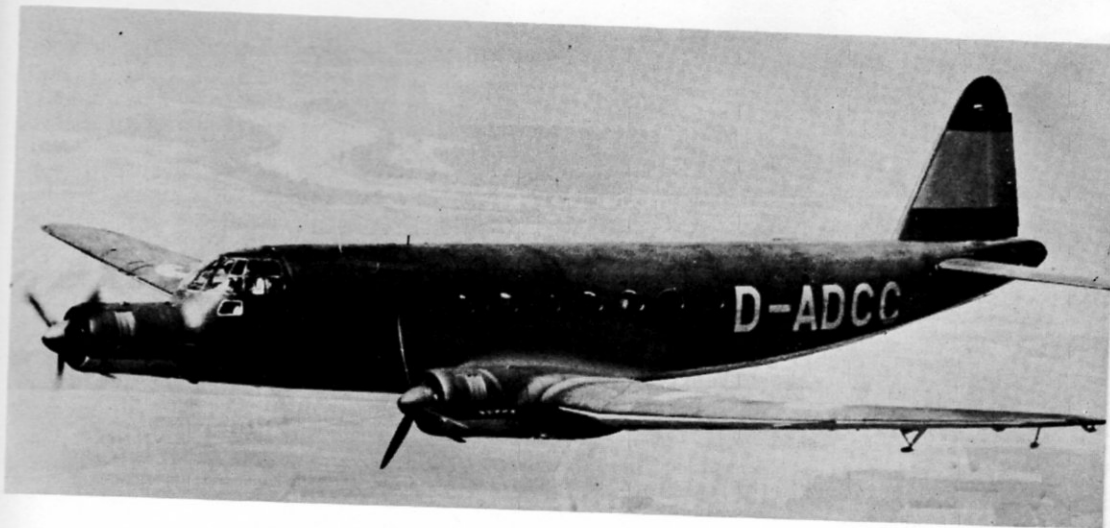
The first Ju 252 prototype on a test flight with stopped port engine Dornier archives
