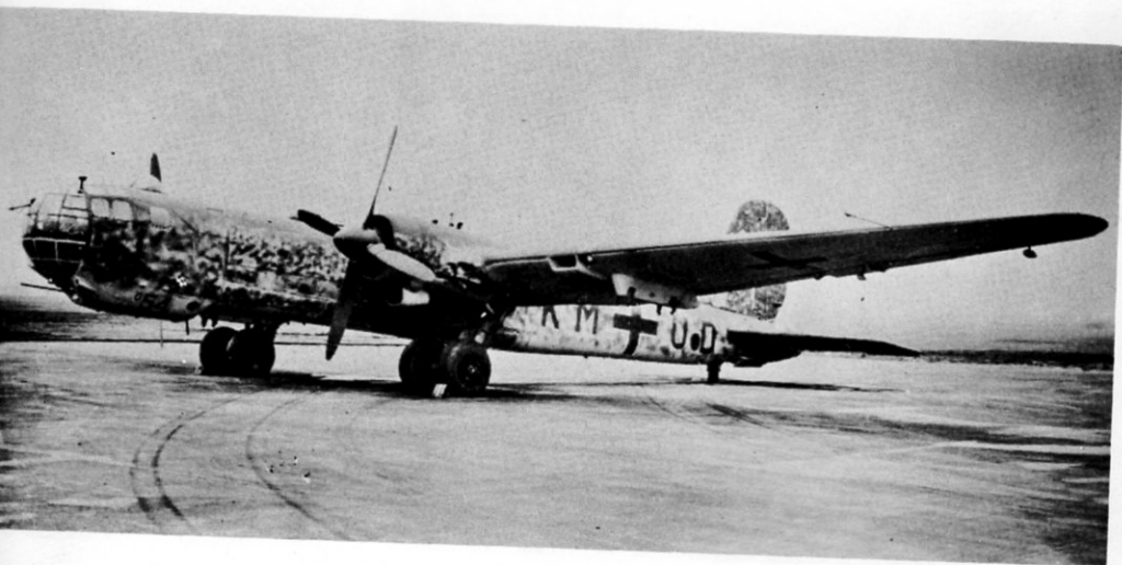
Heinkel He 177A-5/R2 Greif heavy bomber. This version could carry up to three FX 1400 Fritz or Hs 293 guided bombs on external racks Hanfried Schliephake coll.
