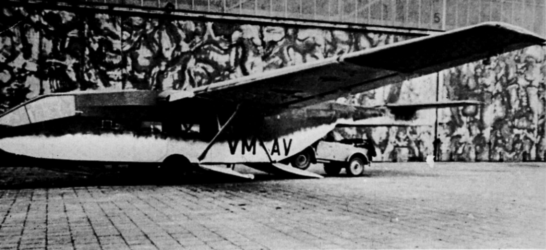
Kalkert Ka 430 cargo glider was a great improvement on the Go 242 but arrived too late and only a small number were completed Hanfried Schliephake coll.
