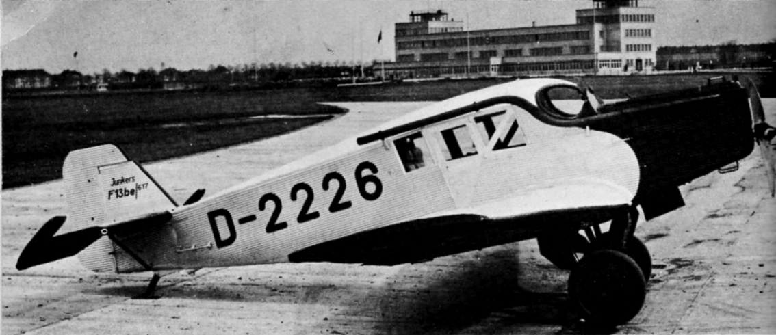
Junkers F 13, the world's first all-metal commercial transport aircraft
